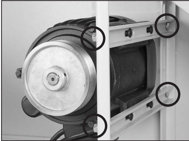
Figure 17. Motor mounting carriage bolts.
